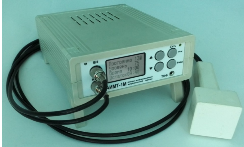
Fig. 1. Device for modeling solar microwave radiation (AIMT-1)
